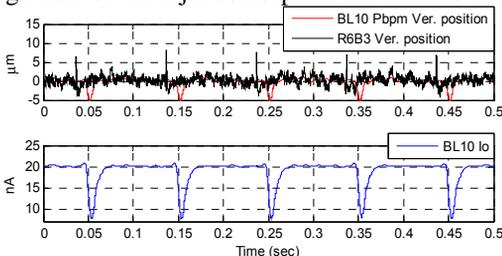
Figure 10: R6BPM3 electron BPM and BL10 PBPM and BL10 Io monitor reading during the injection septum and kicker fired.
