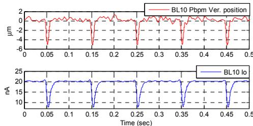
Figure 8: BL10 PBPM and BL10 Io monitor reading during the injection septum and kicker fired.
