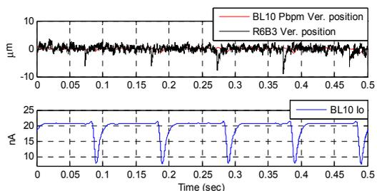
Figure 7: R6BPM3 electron BPM and BL10 PBPM and BL10 Io monitor reading during the injection kickers fired only.
