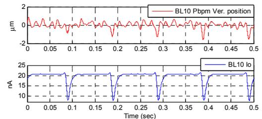
Figure 6: BL10 PBPM and BL10 Io monitor reading during the injection kickers fired only.
