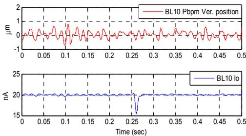
Figure 2: BL10 PBPM and BL10 Io monitor reading during the case of open the transverse feedback system for 3 msec.
