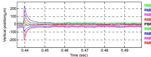
Figure 9: Data form electron BPM and PBPM shown the orbit excursion due to the eddy current induced by the leakage field of the injection septum and kickers fired.
