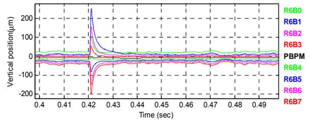
Figure 4: Data form electron BPM and PBPM shown the orbit excursion due to the eddy current induced by the leakage field of the injection septum fired.
