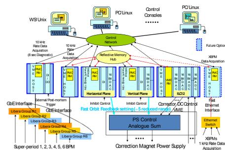
Figure 1: Data acquisition system which is in construction for the RF BPM, PBPM and Io monitors.
