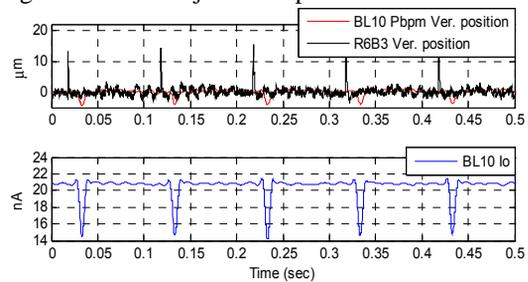
Figure 5: R6BPM3 electron BPM and BL10 PBPM and BL10 Io monitor reading during the injection septum fired only.
