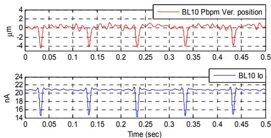
Figure 3: BL10 PBPM and BL10 Io monitor reading during the injection septum fired.
