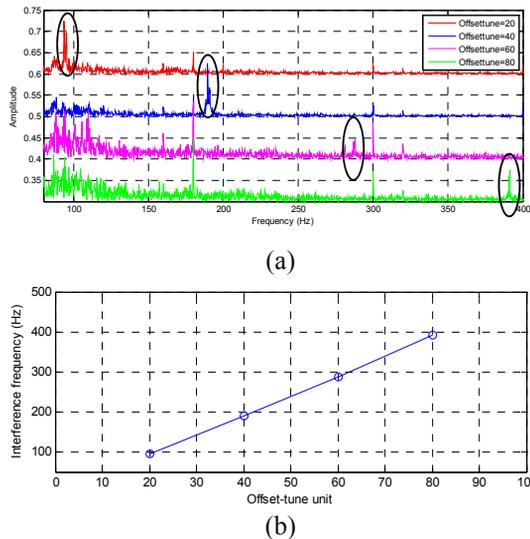
Figure 4: (a) BPM reading spectrum v.s. different offset-tune setting; (b) Offset-tune setting v.s. interference frequency.
