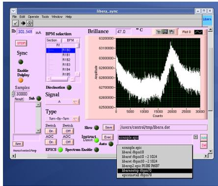
Figure 3: The Libera BPM configuration setup tool.
