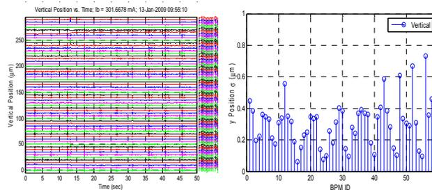
Figure 8: Slow data of vertical position and its rms value.
