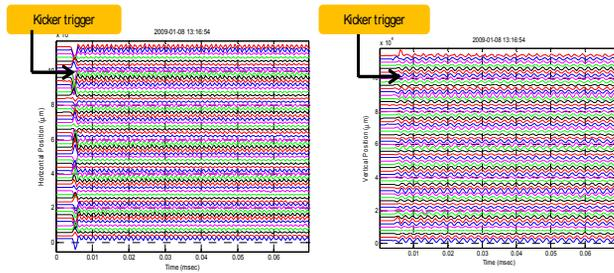
Figure 7: Turn by turn data of vertical and horizontal position. Right figure is horizontal position; left is vertical.
