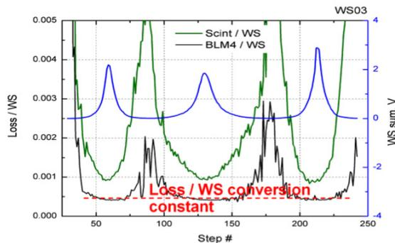
Figure 1: BLM readings normalized over WS signal.
