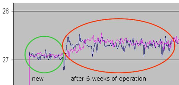
Figure 4: Representative “empty” signal from the first CCD camera, i.e. average over non-illuminated sector of frame, at the start (green circle) and at the end (red oval) of the VIMOS service period. Due to hot pixels the background level shifted just noticeable after irradiation, and fluctuations from frame to frame increased.
