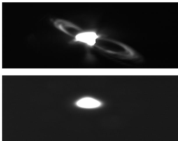
Figure 2: Set-up of the VIMOS camera by means of a special tool with a light emitting diode five years apart. Whereas the top image from the very start of operation features some reflections, nothing of this kind is visible after “seasoning” of the mesh. The absence of reflected light is consistent with the observed decrease in overall signal during the first year of irradiation.
