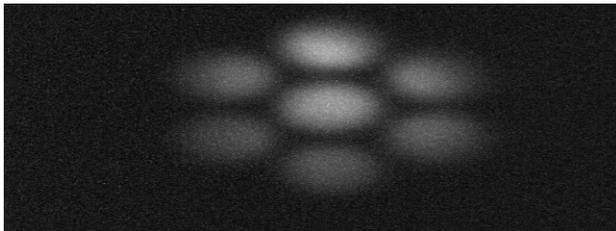
Figure 3: Image obtained through the light guide and with a CCD camera without shielding after 6 weeks of operation during nominal beam conditions at 1350  $\mu$ A.
