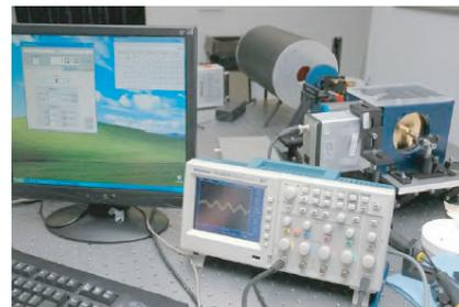
Figure 4: Photograph of the RadiaBeam Terahertz laboratory setup where the interferometer and detector are being tested with a calibrated blackbody source and a 10.6  $\mu\text{m}$  CO<sub>2</sub> laser. The results are compared to the standard Michelson scanning interferometer.
