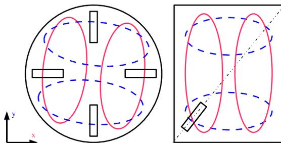
Figure 1: Magnetic fields of the dipole mode in a cylindrical and a square-shaped cavity.
