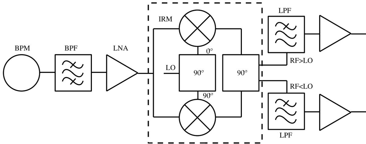
Figure 2: Processing scheme that can be used for separating the signals from a single-coupler CBPM.
