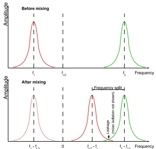
Figure 3: Frequency conversion in the IRM mixer electronics.
