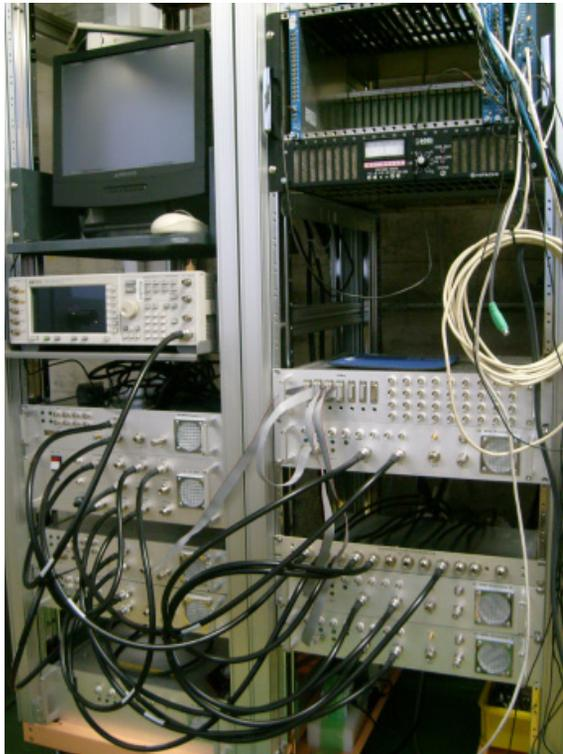
Figure 4: S-band electronics system in a rack at ATF2.
