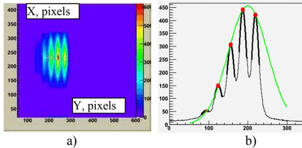
Figure 4: Beam image (a) observed with the multi-pinhole camera and its y-plane projection (b).
