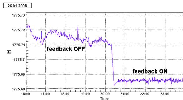
Figure 1: The VEPP-4M guide field stabilization.
