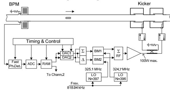
Figure 6: Mode-by-mode longitudinal feedback system.
