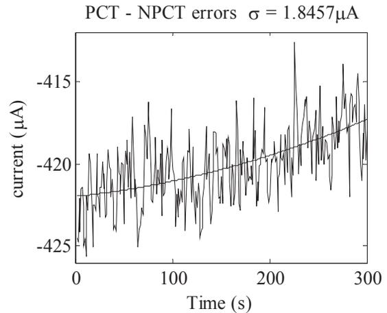
Figure 2: Difference between PCT and NPCT with 500 mA stored. The 420  $\mu\text{A}$  offset can be zeroed out.
