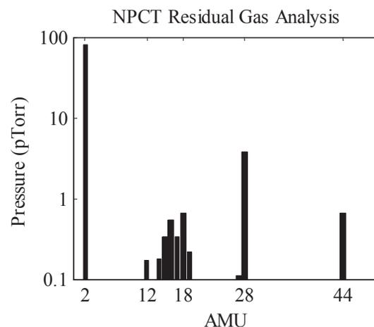
Figure 1: RGA after completion of all vacuum processing.
