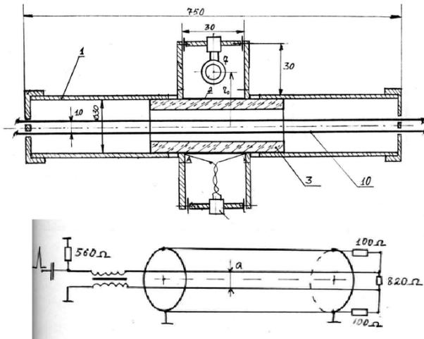
Figure 3: Schematic view of the experimental set-up and electrical diagram of the transmission line. 1- aluminium pipe, 2 – 50 micron stainless steel foil, 3 - Plexiglas foil support, 7 - measuring coil, 10 – two-wire transmission line.
