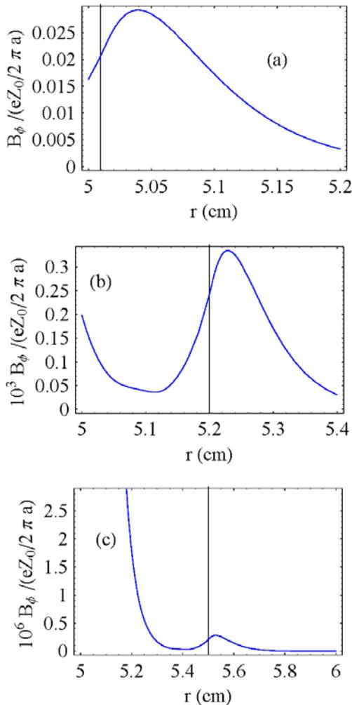
Figure 6: Radial dependence of the  $m=1$  harmonics within the wall for (a)  $\Delta=0.01$  cm, (b)  $\Delta=0.2$  cm, and (c)  $\Delta=0.5$  cm. The vertical line corresponds to the radius of  $a+\Delta$ .
