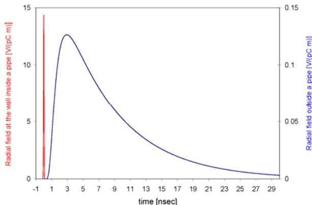
Figure 1: The radial component of the E-field on the inner (red line) and outer (blue line) sides of a beam pipe.
