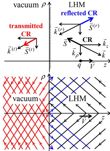
Figure 2: Top: Wave vectors and power flux densities of CR and CTR (reflected and transmitted waves). Bottom: The lines are parallel to the power flux density of CR (black), the reflected wave (blue) and the transmitted wave (red); one can see areas of interference.
