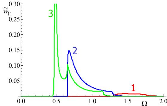
Figure 3: Dependence of the energy spectral density of the first mode in vacuum  $\tilde{w}_{11}$  (normalized with multiplier  $\pi c/4q^2$ ) as a function of the normalized frequency  $\Omega = \omega/\omega_{pe}$  for different values of the radius: 1 –  $a = 1$  cm, 2 –  $a = 2$  cm, 3 –  $a = 3$  cm;  $\beta = 0.5$ ,  $\omega_{pe} = 9$ GHz.
