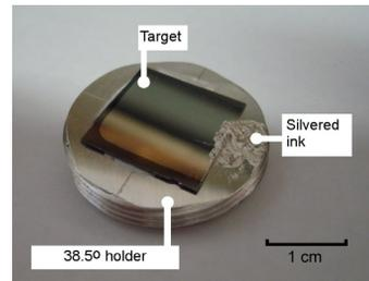
Figure 4: OTR target fixed in the holder.
