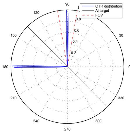
Figure 2: OTR emission of a 38 MeV electron incident on a 45°-inclined perfect conductor. Beam propagation from 0° to 180°.
