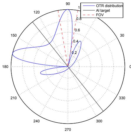
Figure 3: OTR emission of a 1.8 MeV electron incident on a 38.5°-inclined perfect conductor. Beam propagation from 0° to 180°.
