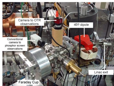
Figure 6: The OTR device in details.
