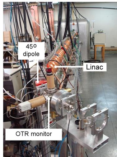
Figure 5: The OTR device installation.
