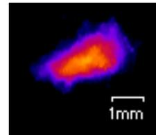
Figure 10: Beam current distribution measured with the OTR monitor.
