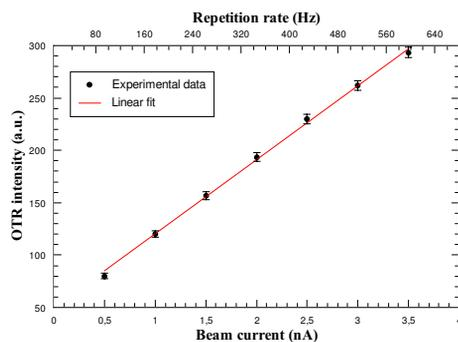
Figure 7: OTR intensity as a function of the beam average current.
