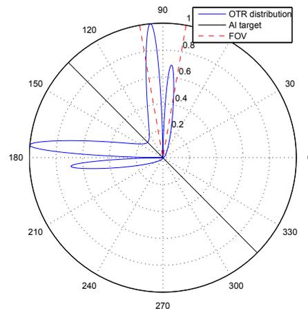
Figure 1: OTR emission of a 5 MeV electron incident on a  $45^\circ$ -inclined perfect conductor. Beam propagation from  $0^\circ$  to  $180^\circ$ .
