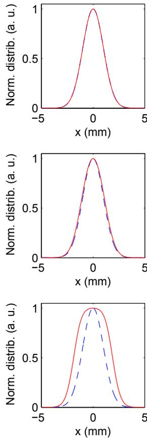
Figure 2: Comparison between the observed beam distribution (continuous line) and the actual beam charge distribution (dashed line) for saturation factor of 1, 10 and 100, respectively.
