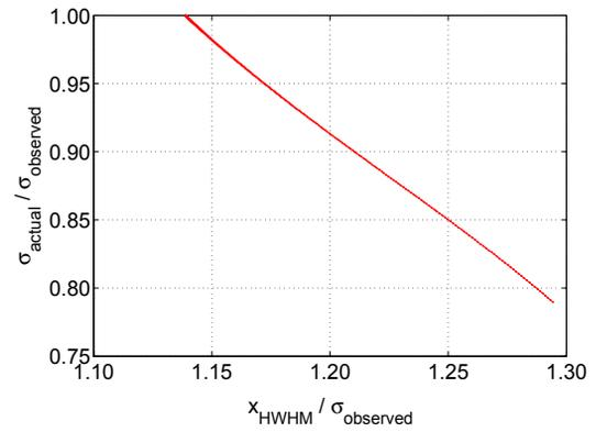
Figure 3: Ratio  $\sigma_{actual}/\sigma_{observed}$  as function of  $x_{HWHM}/\sigma_{observed}$ .
