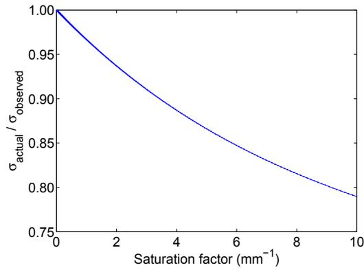
Figure 1: Ratio  $k = \sigma_{actual}/\sigma_{observed}$  as function of saturation factor.
