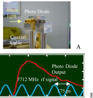
Figure 5: A. EUV in-vacuum photo-diode detection system. B. 60 nm EUV light pulse detected with the PD.
