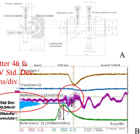
Figure 3: A. Cross-sectional view of the BPM cavity. B. Beam arrival time jitter measured with the BPM intensity cavity. The Std. Dev. of  $0.54\text{mV}$  corresponds to a  $46$  fs jitter (rms). The BPM detection circuit uses the IQ method.
