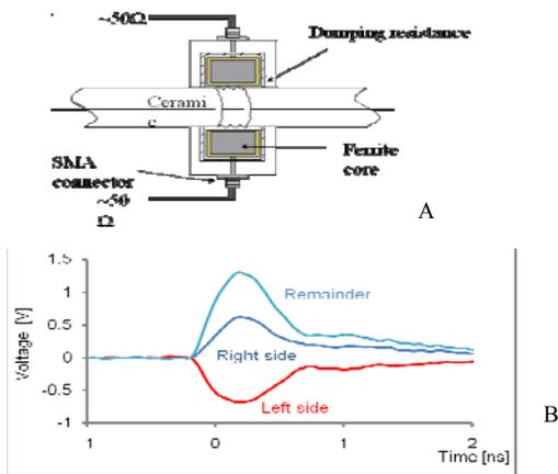
Figure 4: A. Cross-sectional view of the differential output-type CT monitor. B. CT output wave forms induced by the electron beam.
