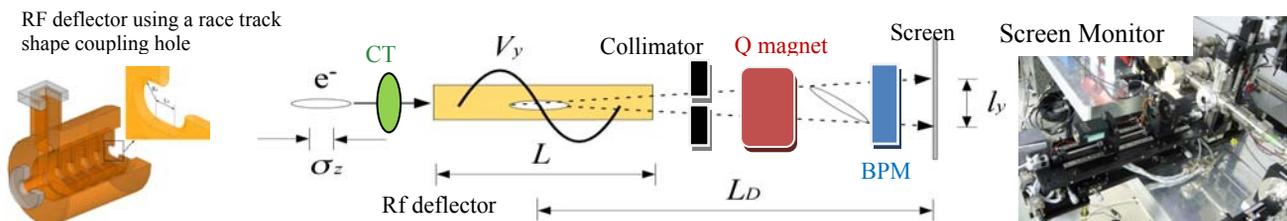
Figure 1: Beam-monitor layout at the rf deflector part (center), RFDEF cavity shape (left), and SCM (right).
