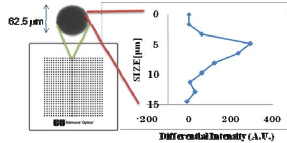
Figure 2: Resolution of the optical system of the SCM. The dot diameter is  $62.5 \mu\text{m}$ . The graph shows that the sharpness (resolution) of the dot edge is about  $4 \mu\text{m}$  (FWHM). The edge sharpness is obtained by differential operation of the dot contrast.
