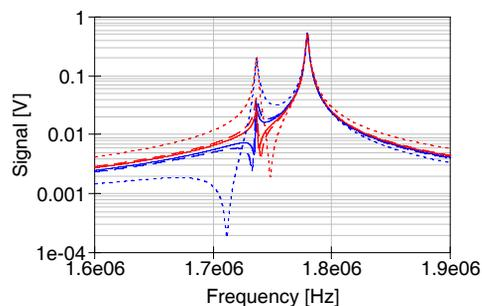
Figure 4: Resulting spectra for different beam displacements (solid line:  $\pm 1$  mm, dashed line:  $\pm 2$  mm, dotted line:  $\pm 10$  mm) for two resonant pick-up electrodes coupled with a parasitic capacitance.
