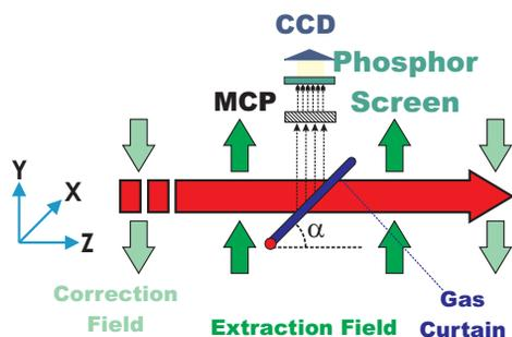
Figure 3: Gas curtain monitor working principle.
