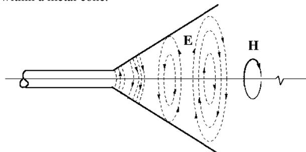
Figure 1: Surface wave evolution inside the launching cone.
