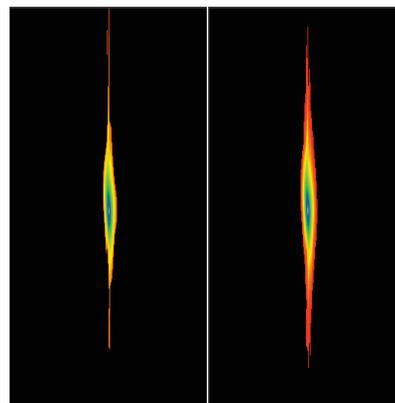
Figure 2: FROG trace from simulation (left) and its reconstruction (right) for the 400 nm case at SPARC.
