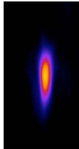
Figure 5: FROG trace of a 400 nm pulse from the Pegasus photoinjector drive laser
