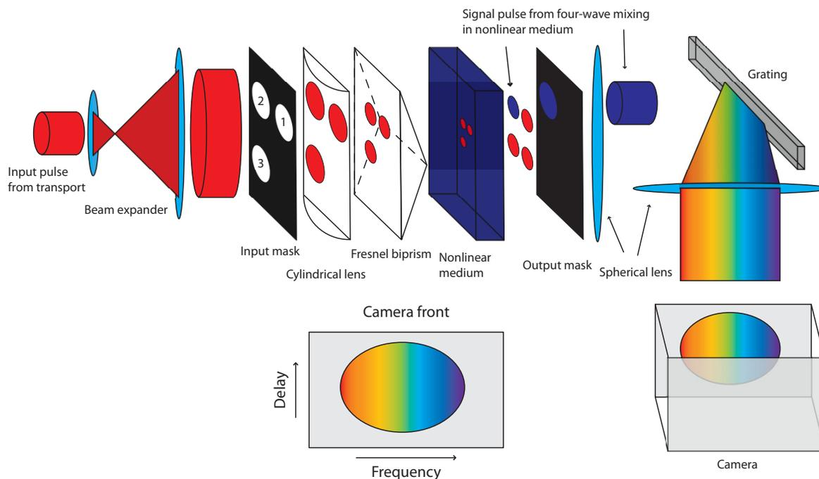
Figure 1: Transient-grating FROG geometry proposed for SPARC FEL as described in Ref. [4].
