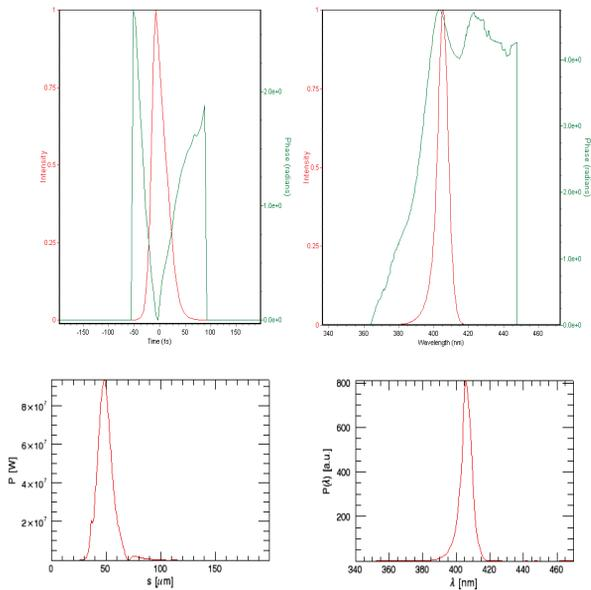
Figure 3: Above: the reconstructed temporal intensity and phase plots (left) and the spectral intensity and phase plots (right). Below: corresponding plots generated by GENESIS simulations.
