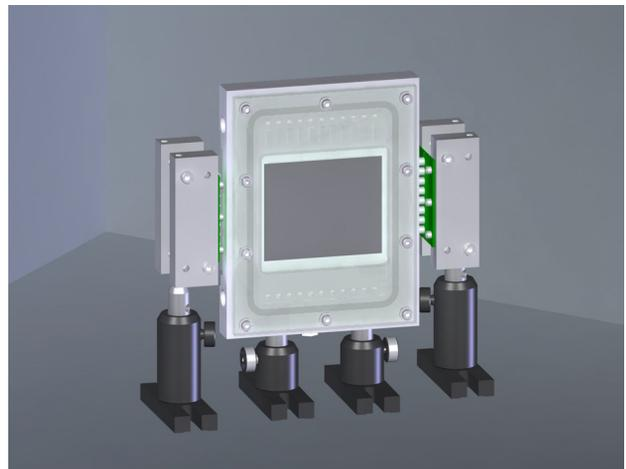
Figure 1: CAD drawing of target holder with redesigned lighting fixture. Two LED bars are located at each side of the holder (in green).
