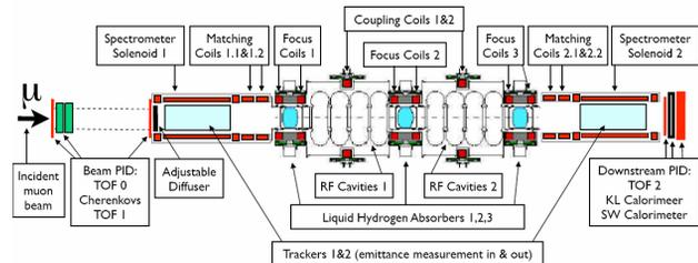
Figure 1: Layout of the MICE experiment with the cooling channel in the center flanked by input and output spectrometers and particle identification detectors.
