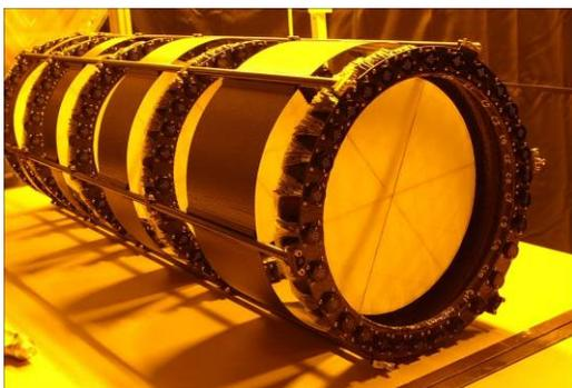
Figure 2: A MICE scintillating fiber tracker.
