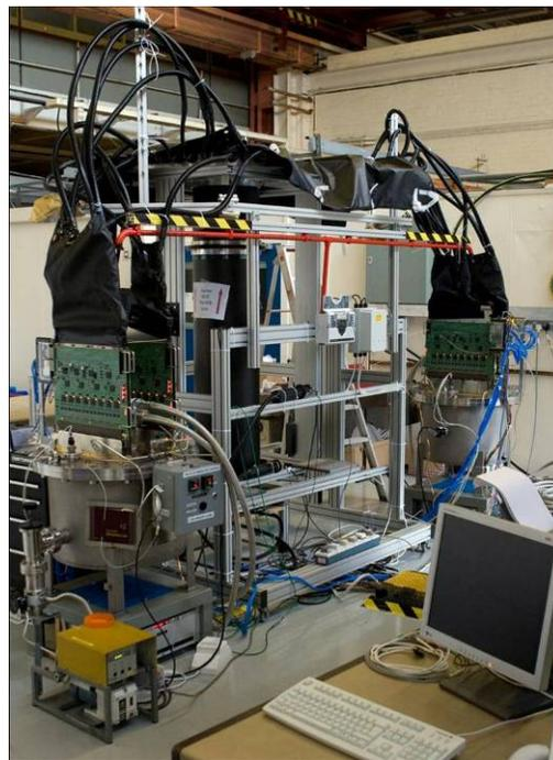
Figure 3: Tracker 1 in the cosmic ray test setup.
