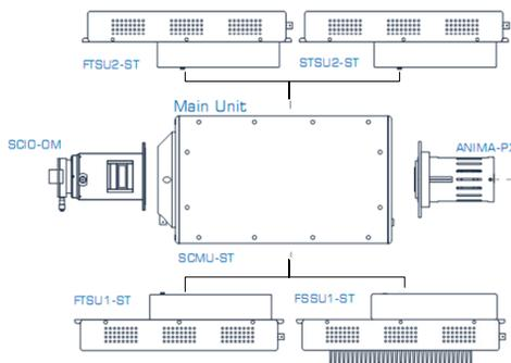
Figure 4: The streak camera main modules.
