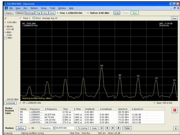
Figure 8: the measurement of synchrotron frequency with multi-bunch.
