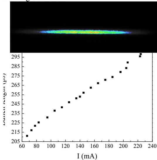
Figure 6: The streak image (up) and the bunch lengthening (down).
