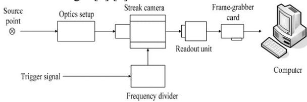
Figure 2: The system functional diagram.
