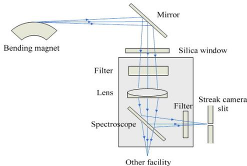
Figure 3: The synchrotron light extracting setup.
