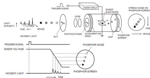
Figure 1: The operating principle (up) and timing (down) of the streak camera.
