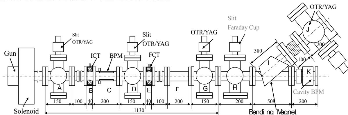
Figure 1: Layout of Beam Diagnostic for High-Brightness Injector in HLS.
