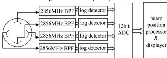
Figure 7: Block Diagram of Log-Ratio Position Signal Processing Module
