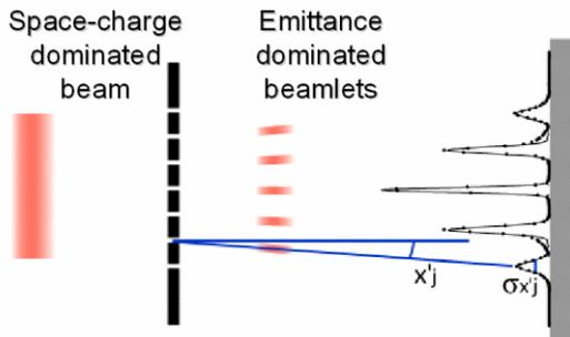
Figure 3: Schematic Diagram of Space Charge Dominated Beam Separated into Beamlets by Multi-slits
