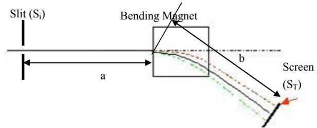
Figure 4: Schematic Diagram of Energy and Energy Spread Measurement
