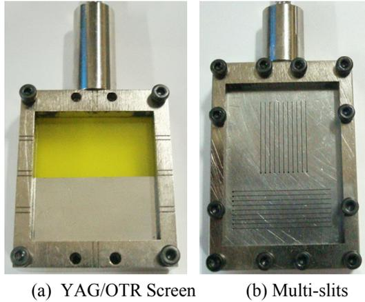
Figure 2: Outline of YAG/OTR Screen and Multi-slits. (a) Top of Left Photo is YAG Screen; While Below is OTR Screen. (b) Top of Right Photo is for Vertical Emittance Measurement; While Below is for Horizontal Measurement.
