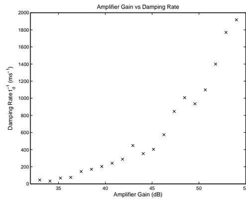
Figure 5: Mode 360 Damping Rate vs Amplifier Gain. The total beam current is 80 mA, evenly filled into 155/360 buckets.
