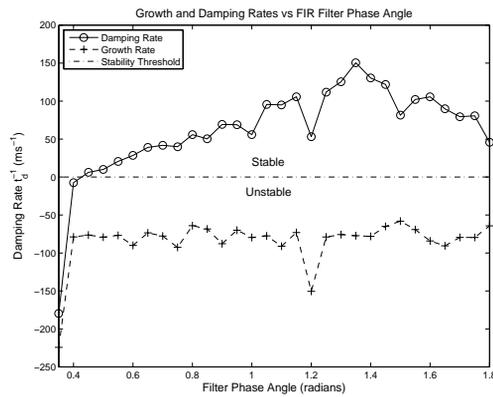
Figure 4: Mode 360 damping rate versus the Finite Impulse Response Filter Angle. It is important that the final corrective pulse placed onto the beam by the kickers is a sinusoid phase shifted by  $\pi$  radians from the beam motion at the kickers.
