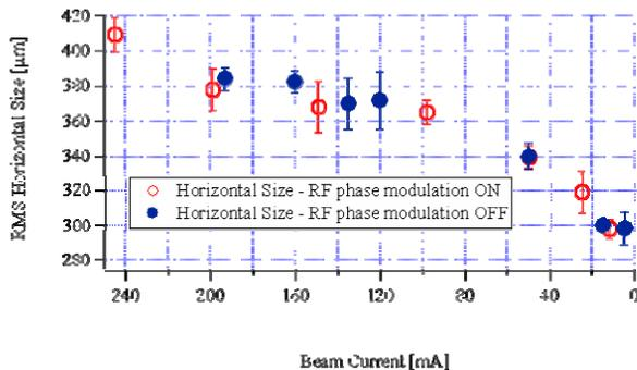
Figure 3: Beam horizontal dimension dependence on the beam current. The increased energy spread caused by the normal conducting RF cavities probably is causing it rather than the RF phase modulation.
