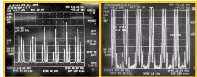
Figure 1: Typical harmless horizontal instability present at the end of the beam accumulation (right). Strong instability in both plans responsible for a 70 mA beam loss in the low energy ramp.
