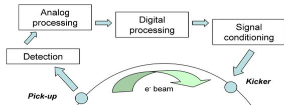
Figure 5: Multi bunch feedback system block diagram.
