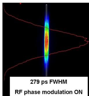
Figure 4: FWHM longitudinal beam size at high current.
