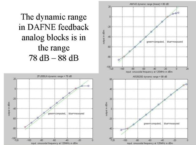
Figure 1: Dynamic range in DAFNE analog transverse feedback modules.
