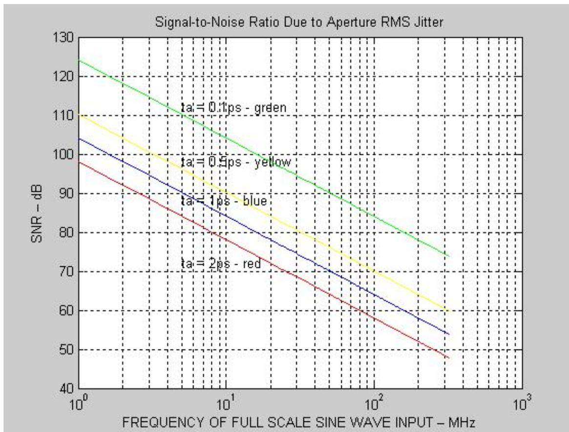
Figure 2: Signal to Noise ratio Due to aperture RMS jitter: at 250 MHz with 0.5 ps jitter the ratio is 60 dB.
