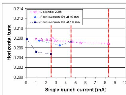
Figure 8: Measured horizontal single bunch detuning and TMCI threshold. No in-vacuum undulators (magenta). 4 in-vacuum undulator gaps closed to 10 mm (light blue) and 5.5 mm (dark blue).
