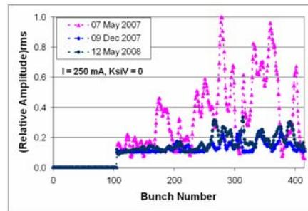
Figure 6: Oscillation amplitude along a bunch train at 250 mA in  $\frac{3}{4}$  filling with zero chromaticity, measured with feedback switched off. Different colors correspond to measurement done at different times.
