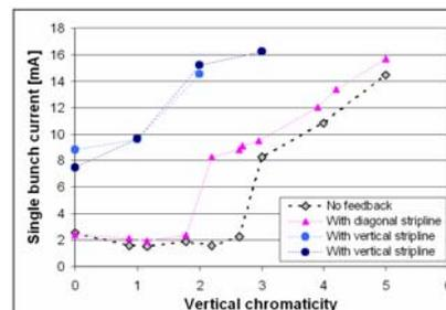
Figure 3: Attained performance of the vertical stripline in single bunch in comparison with previous results.
