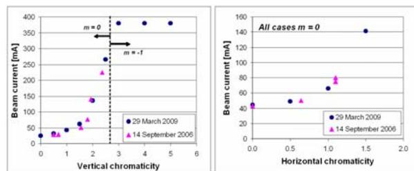
Figure 7: Vertical (left) and horizontal (right) threshold current measured in  $\frac{3}{4}$  filling as a function of chromaticity. Different colors correspond to measurement done at different times.
