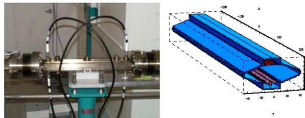
Figure 2: Picture of the vertical stripline installed in the ring (left) and a sketch of its structure (right).
