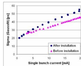
Figure 9: Bunch lengthening measured before (magenta) and after (dark blue) installation of the 2<sup>nd</sup> RF unit.
