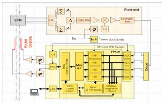
Figure 1: Layout of the SOLEIL feedback chain.
