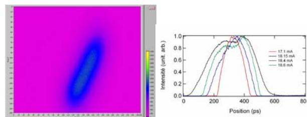
Figure. 10: Observed microwave instability after installation of the 2<sup>nd</sup> RF unit. Left: An X-ray pinhole image. Right: Longitudinal profile measured with a streak camera.
