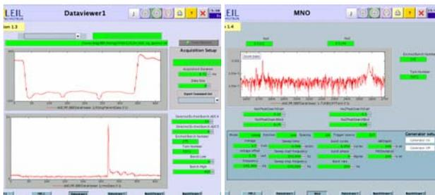
Figure 5: Left: Online acquisition showing the  $\frac{3}{4}$  filling pattern (upper) and oscillation amplitude (lower). The peak seen represents the excited bunch for the tune measurement. Right: Tune spectrum of the excited bunch.
