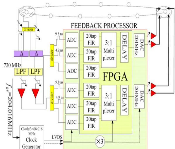
Figure 5: Overview of the HLS digital transverse bunch-by-bunch feedback system.
