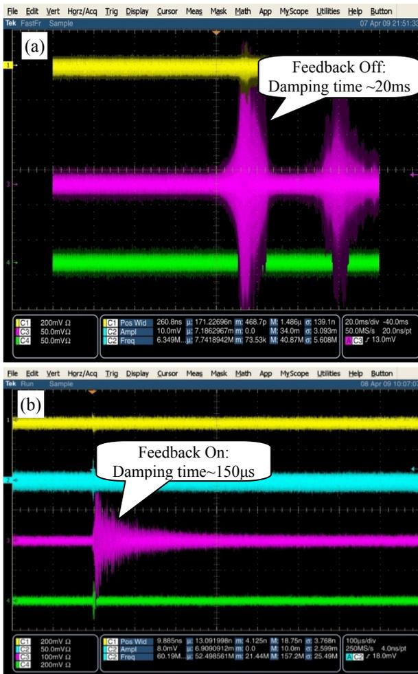
Figure 6: The damping time due to injection bump excitation was decreased by feedback system. (a) damping time was about 20ms due to injection bump excitation; (b) damping time was decreased to about 150µs by feedback system.
