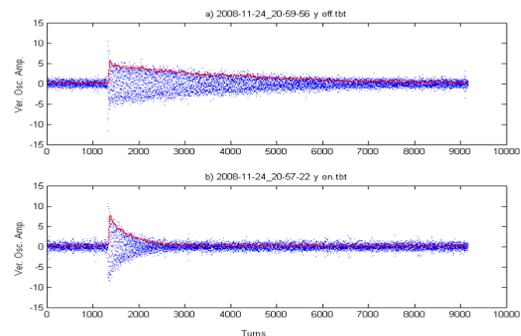
Figure 2: Turn by turn beam tracking of vertical direction at 200MeV injection when feedback system is off and on.
