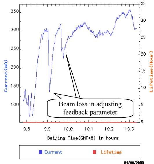
Figure 7: The injecting accumulating beam current curve in commissioning of digital TFB system.
