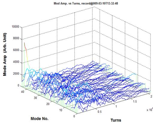
Figure 3: Mode tracking with feedback off.
