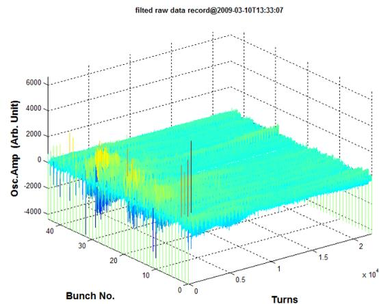
Figure 6: Bunch tracking with feedback off.
