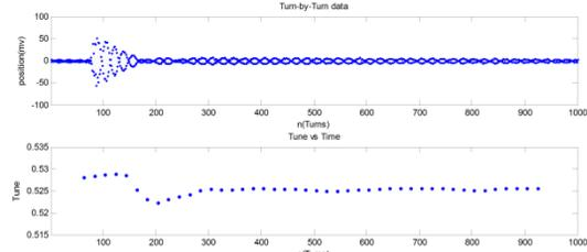
Figure 2: Turn by turn tracking of horizontal direction at 200MeV injection with octopole magnet on, low part show the transient tune.
