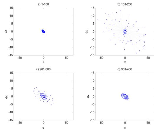
Figure 3: Phase space tracking of horizontal direction at 200MeV injection with octopole magnet on.
