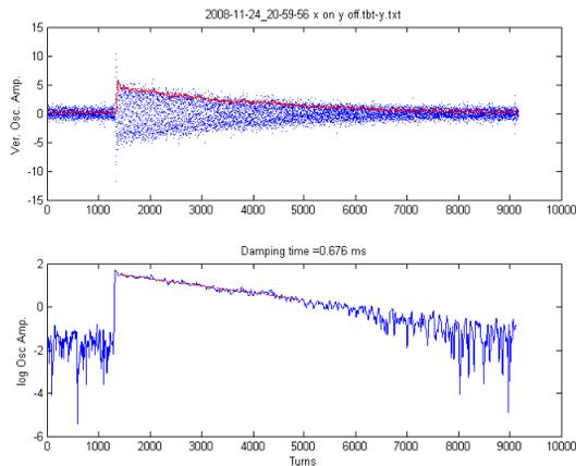
Figure 4: Turn by turn tracking of vertical direction at 200MeV injection status with feedback off. a) Turn by turn position, the red line is envelope. b) Logarithm arithmetic envelope of position, the red line is linear fitting for damping rate.
