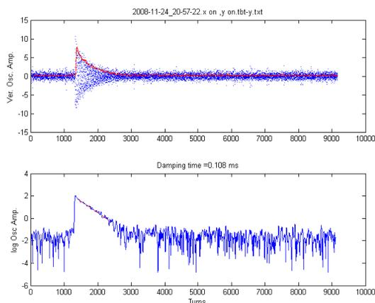
Figure 5: Turn by turn tracking of vertical direction at 200MeV injection status with feedback on. a) Turn by turn position, the red line is envelope. b) Logarithm arithmetic envelope of position, the red line is linear fitting.
