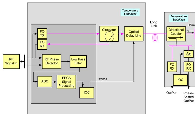
Figure 1: Phase Stable Link block diagram showing the transmitter, receiver, and optical components. The pink lines are optical fiber lines.
