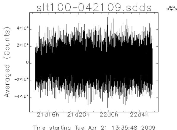
Figure 4: Closed loop phase detector output over a 14-hour run. The peak deviation corresponds to about +/- 0.2 degrees of phase.
