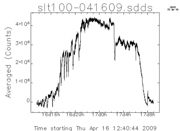
Figure 3: Open loop phase detector output for an overnight. The deviation corresponds to about 10 degrees of phase. The temperature varied by about 4.5 degrees.
