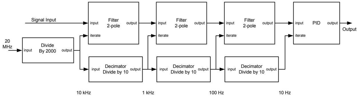
Figure 2: Block diagram of FPGA logic showing 3 2-pole filters with decimators.
