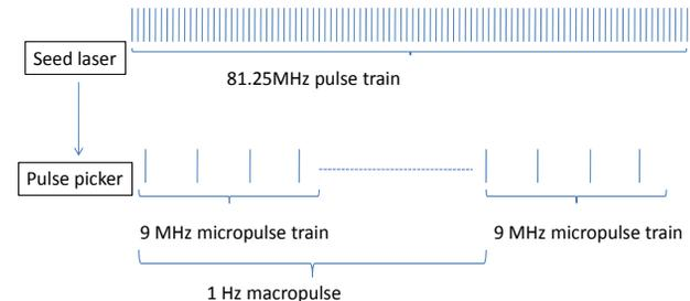
Figure 1: Schematic of the micropulse train and macropulse train at A0.
