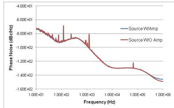
Figure 4: Phase noise plots with and without amplifier.
