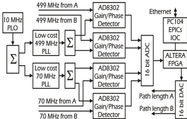
Figure 2: MO diagnostic block diagram.
