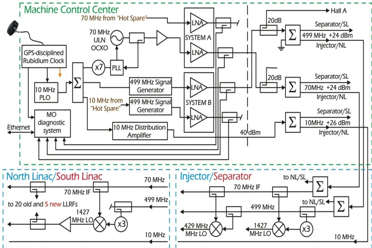
Figure 1: Block diagram of the MO system.
