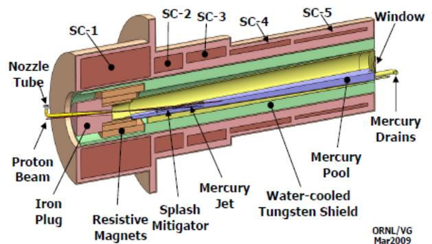
Figure 4: Hg-jet target concept studied in MERIT.
