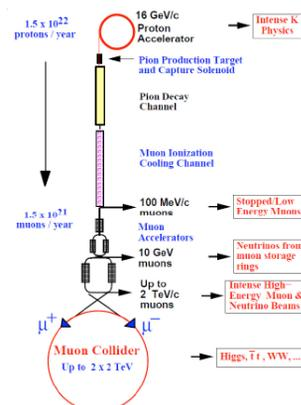
Figure 1: Schematic of MC subsystems.
