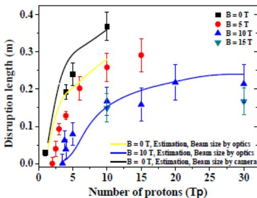
Figure 5: Disruption length vs. proton intensity.
