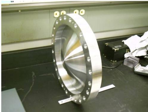
Figure 9: Thin aluminum window used for liquid-hydrogen absorber. The window and flange are machined at the University of Mississippi from a single disk, whose thickness in the center is reduced to 175  $\mu\text{m}$ .
