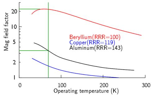
Figure 8: Relative increase in allowable axial field vs. initial temperature for Copper, Aluminum, and Beryllium.
