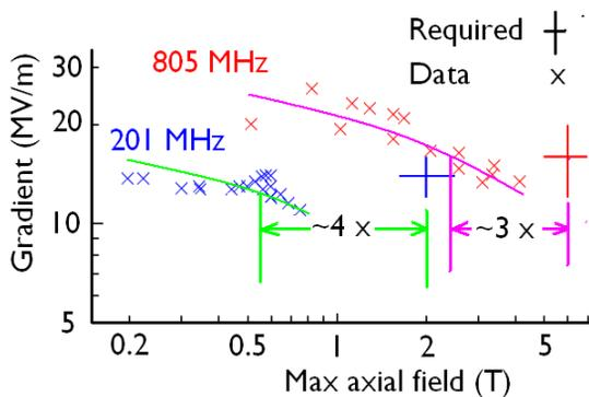
Figure 7: Observed breakdown gradients vs maximum axial fields on cavities, together with approximate required gradients: 201 MHz in blue, 805 MHz in red.
