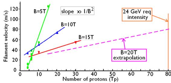
Figure 2: MERIT observed filament velocities vs. proton intensity at B=5, 10, 15 T, & dashed extrapolation to 20 T.
