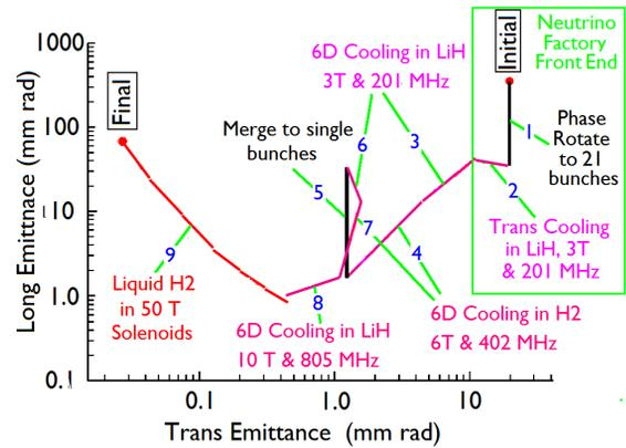
Figure 3: Transverse vs. longitudinal emittances before and after each stage.
