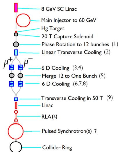
Figure 1: Schematic of Muon Collider components.
