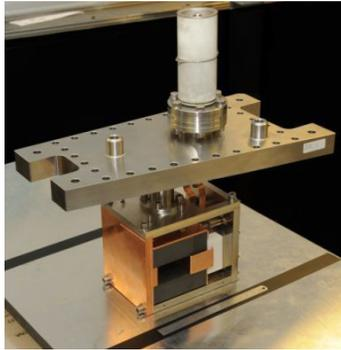
Figure 7: Photograph of the kicker magnet prototype with top-plate and coaxial feed-through; note the 15 cm ruler.
