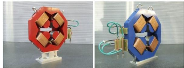
Figure 3: The EMMA prototype magnets (F left, D right).
