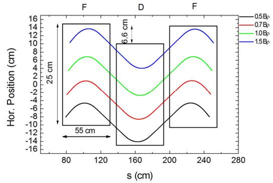
Figure 8: Current layout of PAMELA lattice triplet, showing beam trajectories.
