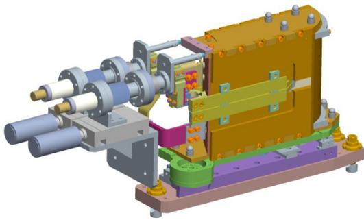
Figure 6: CAD model of the EMMA septum magnet outside its vacuum chamber.
