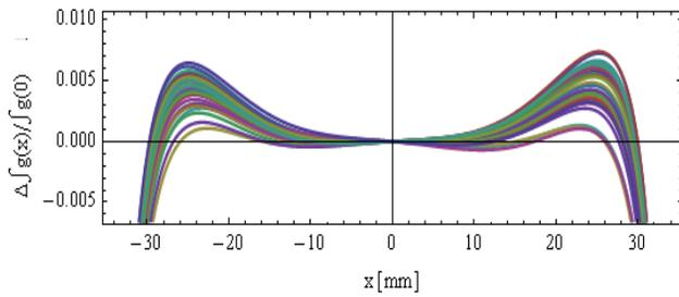
Figure 4: The gradient quality of 34 production Fs, expressed as  $\Delta jg(x)/jg(0)$ .
