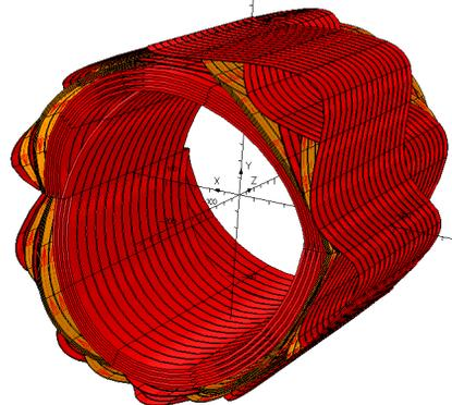
Figure 9: The arrangement of multiple counter-wound helical super-conducting coils to generate the required four field components in the PAMELA combined function magnets.
