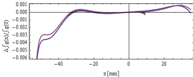
Figure 5: The gradient quality for 2 production Ds, expressed as  $\Delta jg(x)/jg(0)$ .
