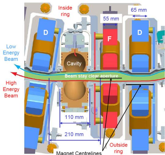
Figure 2: Plan view of an EMMA quadrupole doublet located to the right of an r.f. cavity, showing positions of clamp-plates and trajectories of the circulating beams.
