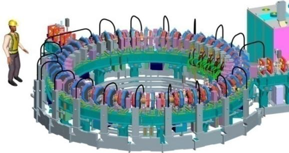
Figure 1: The EMMA lattice containing 42 F and 42 D magnets.
