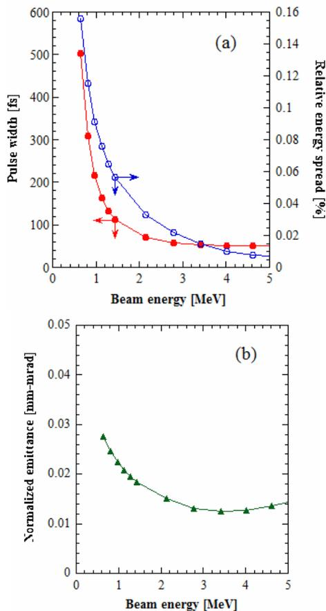
Figure 2: Simulation results of pulse width, energy spread and transverse emittance versus beam energy.
