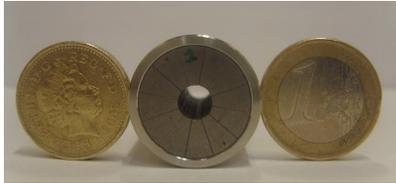
Figure 3: One of the quadrupoles compared with a 1 euro and 1 pound coin.
