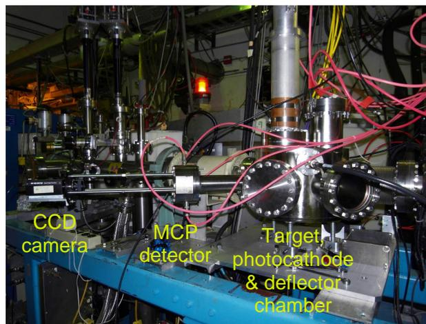
Fig. 2. General view of the X-BLD incorporated into the ATLAS beam line.
