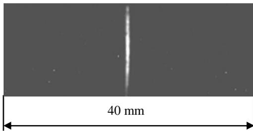
Fig. 4. Image of photoelectrons on the phosphor screen without RF deflection.
