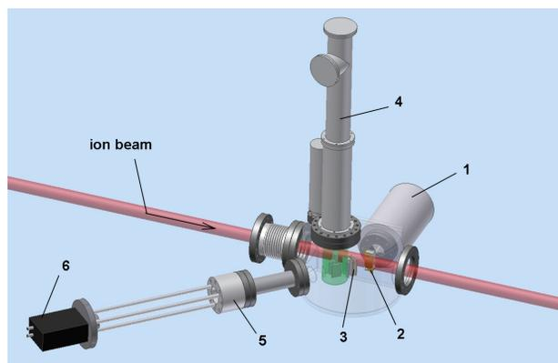
Fig. 3. 3D model of the X-BLD: 1 – target translator, 2 – Cu target, 3 – CsI photocathode, 4 – RF deflector, 5 – dual MCP – phosphor screen, 6 – CCD-camera.
