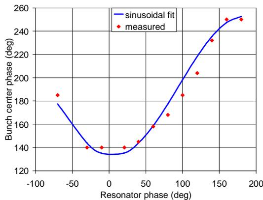
Fig. 6. Bunch center phase as a function of the RF phase in the last RF cavity (97 MHz) of the booster.
