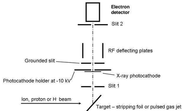
Fig. 1. General layout of the X-BLD.
