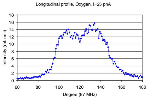
Fig. 5. Typical longitudinal profile of the 1.6 MeV/u oxygen beam.
