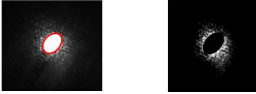
Figure 1: Left: picture of HeNe laser imaged onto a DMA with a defined core specified by the red oval overlay; right: same picture with core light removed.
