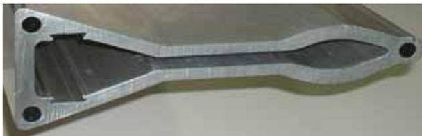
Figure 4: NSLS-II Multipole vacuum chamber.
