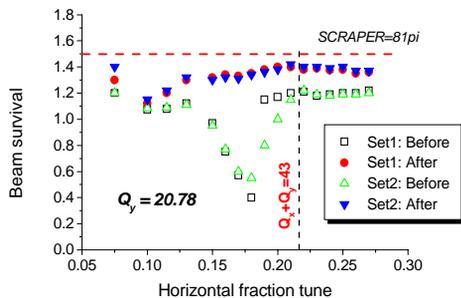
Figure 4: Simulated 'beam survival' at the MR collimator with the physical aperture of  $81 \pi$ .mm.mrad for different horizontal betatron tunes ( $Q_y=20.78$ ) before and after the correction of the linear coupling resonance.
