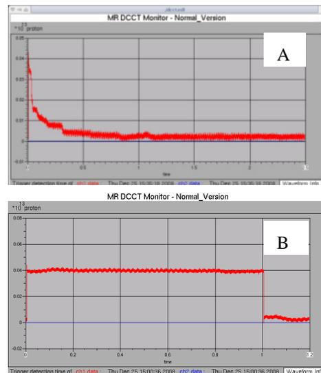
Figure 3 (A,B): The measured changing the beam intensity during the injection process for the MR operation (RUN20) for different ‘bare’ working points: on the [1,1,43] resonance (A) and away from the [1,1,43] resonance (B).
