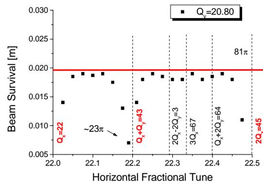
Figure 1: Simulated ‘Beam Survival’ at the MR collimator with the acceptance of  $81\pi$  mm.mrad as function of the horizontal betatron tune ( $Q_y=20.80$  fixed).
