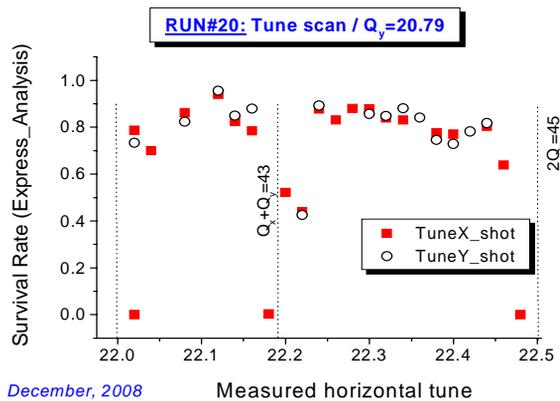
Figure 2: ‘Survival Rate’ of the beam at the injection energy for different values of the horizontal betatron tunes, obtained during the MR commissioning RUN#20 in December 2008.
