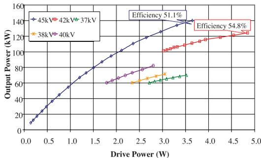
Figure 5: Transfer curve of the ERL injector klystron.
