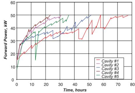
Figure 6: Input coupler processing under full reflection (cavity detuned) up to 50 kW. Shown is the maximum forward power per twin-coupler vs. of processing time (pulsed operation with 2 ms pulse length and 20 ms repetition rate).
