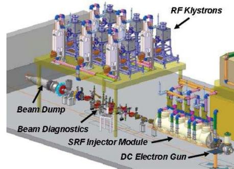
Figure 1: Layout of the ERL injector prototype.
