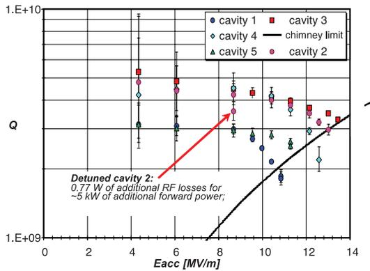
Figure 8: Intrinsic quality factor of the five 2-cell injector SRF cavities as a function of accelerating field gradient at 2K. Also show is the 1 W/cm<sup>2</sup> heat flux limit for the LHe in the chimney connecting the LHe tank around the cavity to the 2K-2 phase LHe supply line.
