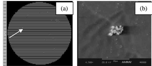
Figure 3: (a) Field emitters revealed by scanning a high-voltage tip over a niobium surface electropolished together with a 9-cell cavity. (b) SEM image of the field emitter (indicated by arrow in Fig. 3a); EDX analysis indicates no foreign elements except niobium and oxide.
