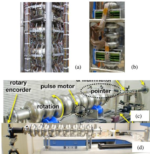
Figure 5: T-mapping systems at KEK (a) and JLab (b) and optical inspection tools at KEK (c) and JLab (d).
