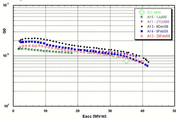
Figure 1: Performance of 5 cavities manufactured by one vendor and EP processed and tested recently at JLab. Error bars are not shown for clarity.
