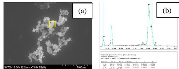
Figure 4: (a) A cluster of Nb<sub>x</sub>O<sub>y</sub> granules with non-uniform S distribution. (b) EDX analysis shows detectable S in the boxed region in Fig. 4a; no detectable S outside the boxed region.
