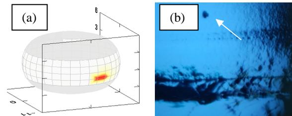
Figure 6: T-mapping and optical inspection of AES5 quench limited at 20 MV/m after the first-pass EP processing. (a) Quench location determined as a “hot spot” near the equator weld of cell #3. (b) The circular defect (indicated by arrow), 700  $\mu\text{m}$  in diameter, 14 mm away from the weld seam, observed on the RF surface at hot spot location.
