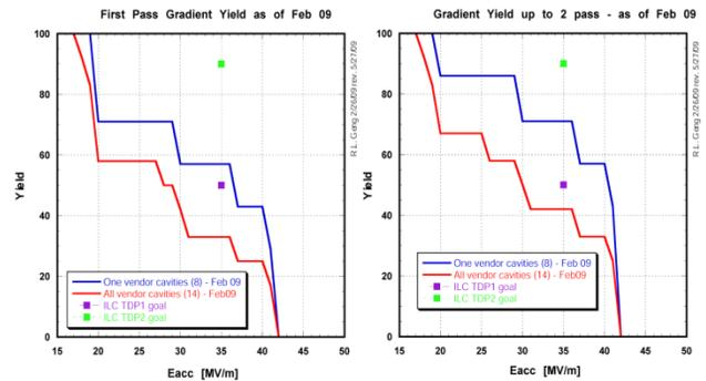
Figure 7: First-pass and second-pass gradient yield based on 14 cavities built by various manufactures (8 from a European vendor, 4 from a US vendor, 1 from a Japan company and 1 from Jefferson Lab) processed and tested at JLab as of February 2009.
