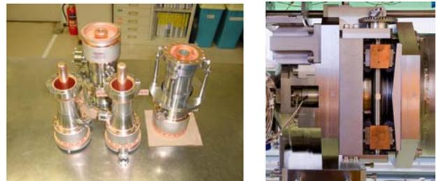
Figure 3: Two pairs of input couplers with a cold and a warm rf window [6], (left), and a frequency tuning system, [7], (right).
