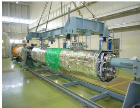
Figure 7: Insertion of an assembled cold mass into a vacuum vessel.
