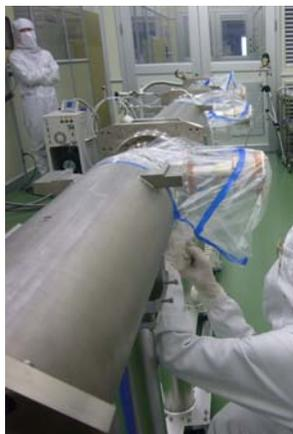
Figure 5: String assembly in a class-10 clean room (left) and vacuum leak-check in a class-1000 clean room (right).
