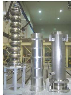
Figure 4: A Tesla-like 9-cell cavity (left), a magnetic shield (central) and a titanium helium vessel (right).
