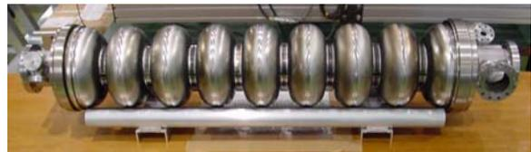
Figure 1: A Tesla-like 9-cell niobium cavity, [1 and 2].
