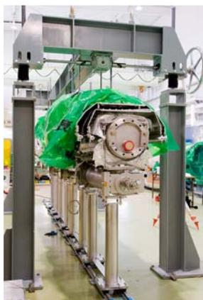
Figure 6: Alignment of four cavities (left) and hanging the string cavities on a GRP (right).
