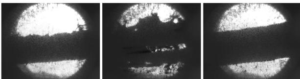
Figure 6: A proton beam/jet interaction as viewed in viewport 3: Left: Image of the jet before interaction; Middle: Image of the interaction aftermath; Right: Image of the reformed jet stream.
