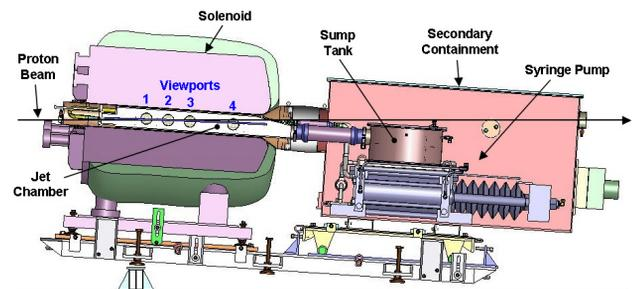
Figure 4: Cutaway side view of the MERIT experiment.
