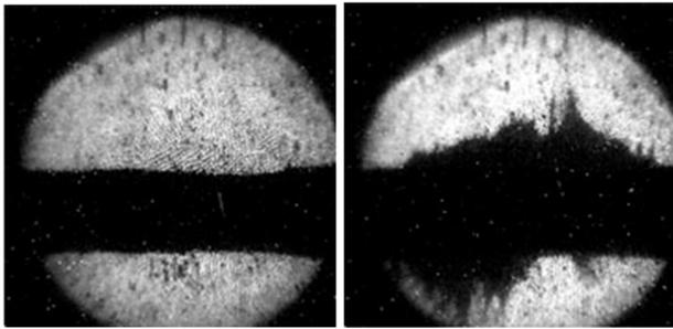
Figure 8: The proton beam/jet interaction of Fig. 6 as viewed in viewport 2: Left: Before interaction; Right: 350  $\mu$ s after proton beam arrival.
