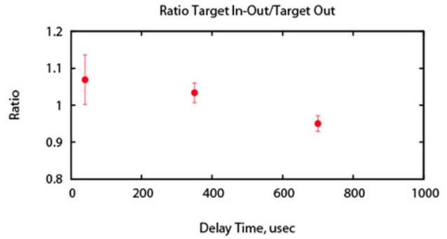
Figure 12: The probe/pump ratio for target-related particle production as a function of delay of the probe bunches.
