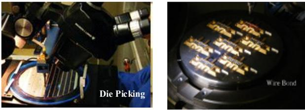
Figure 3 : manufacturing phases
