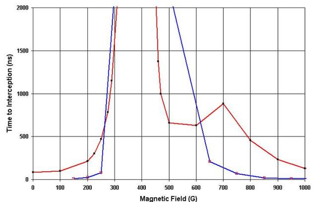
Figure 11: Stability of a 2-cavity PCM system (2D-red curve, 3D-blue curve).
