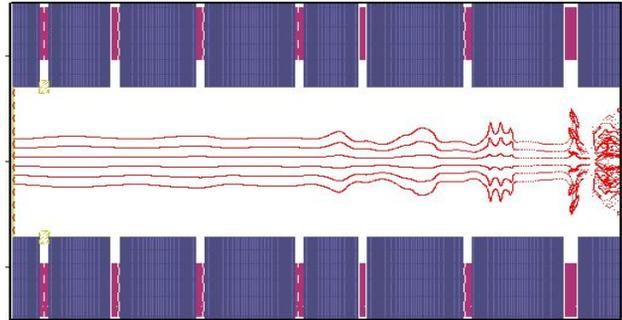
Figure 10: 10 MW 390 G-780 G solenoid design.
