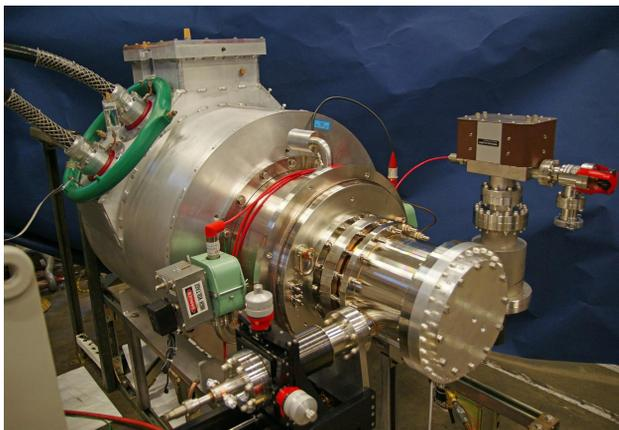
Figure 12: BSD mounted to small oil tank and connected to modulator.
