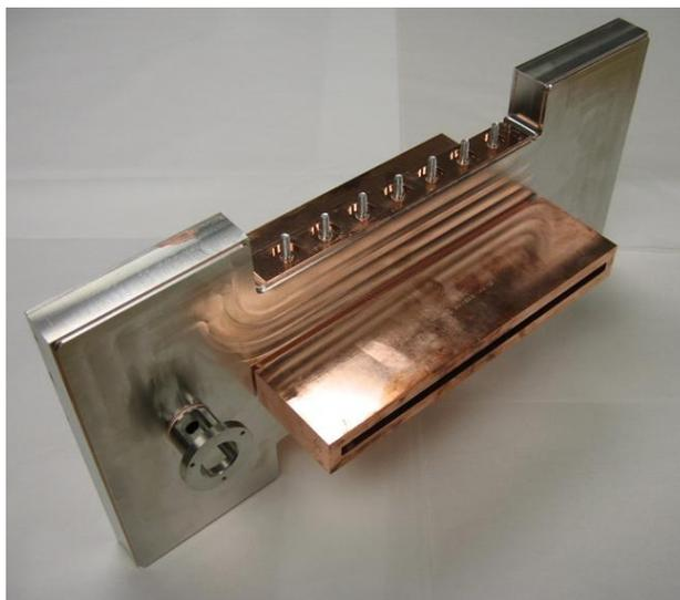
Figure 7: Cavity 2 with loading and sensor port.
