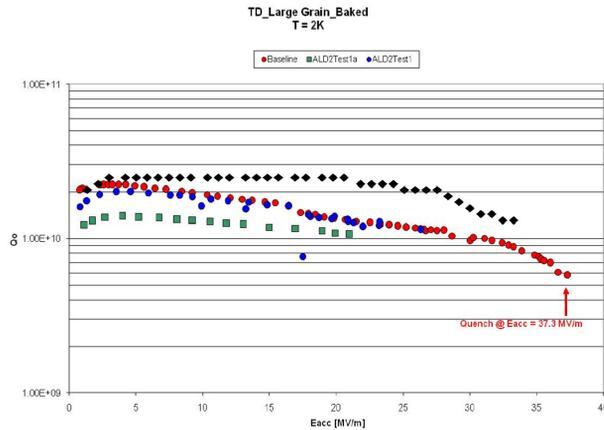
Figure 1: Tesla/ILC shape 1.3GHz cavity. RRR> 300, large grain Nb from Tokyo-Denkai. BCP and in-situ mild baked. In Bleu after the first coating with 10 nm of Al<sub>2</sub>O<sub>3</sub> and 3 nm of Nb<sub>2</sub>O<sub>5</sub>. In green after the second HPR. In Black after the second ALD coating with 5 nm of Al<sub>2</sub>O<sub>3</sub> and 15 nm of Nb<sub>2</sub>O<sub>5</sub>.
