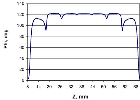
Figure 7: Phase advance/cell along the structure.
