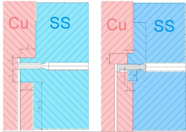
Figure 6: Copper enhances heat transfer.
