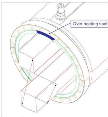
Figure 1: Over heating spot.
