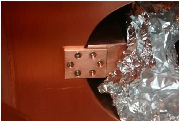
Figure 5: Implementation of a short circuit.
