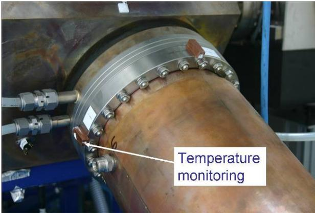
Figure 7: Temperature measurement.
