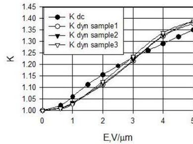
Figure 2: Example of DC tunability  $K_{dc}$  and dynamic (short  $\sim$ ns pulse) tunability  $K_{dyn}$  for different compositions of BST(M) ferroelectric. Note that for a bias field  $> 3 \text{ V}/\mu\text{m}$  ( $30 \text{ kV}/\text{cm}$ )  $K_{dyn} > K_{dc}$ .
