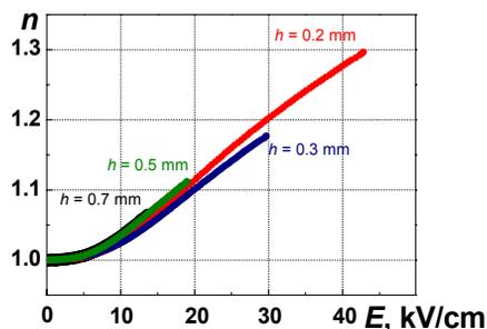
Figure 1: BST(M) ferroelectric tunability dependence on the DC field magnitude.
