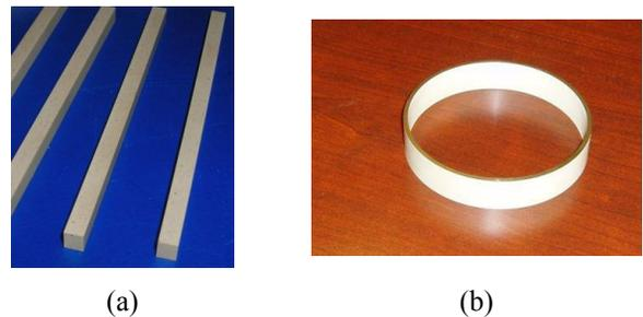
Figure 3: (a) BST(M) ferroelectric bar samples fabricated for a 1.3 GHz planar phase shifter; (b) BST(M) ferroelectric ring sample. The ring diameter is 110 mm, and its thickness is 2.8 mm.
