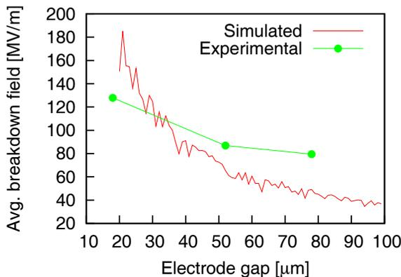
Figure 3: The model predicts that the average breakdown field will drop when the electrode gap is increased, an effect of the electrode geometry (red line). Similar behaviour is observed in experiments (green dots).
