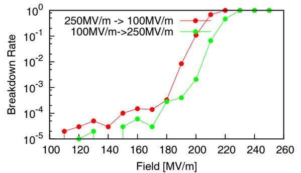
Figure 1: The breakdown rate as a function of field  $V/d$ . The electrode gap is set to  $20\ \mu\text{m}$  and 100 000 breakdown attempts are simulated for each field value. The red curve is for a downwards field scan, the green curve for an upwards scan
