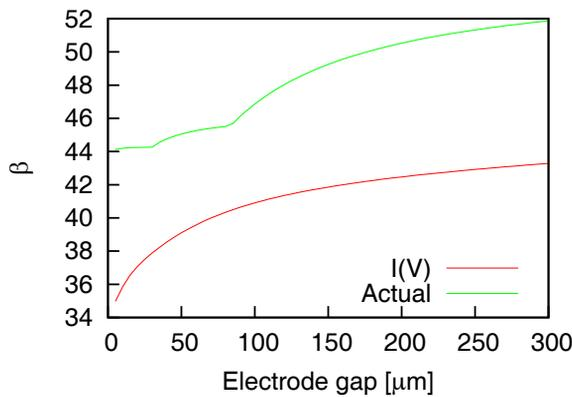
Figure 2:  $\beta$  dependence on electrode gap spacing for a field emission experiment, simulated as a measurement of current as a function of voltage (red curve), where  $\beta$  is calculated assuming a field  $V/d$ . The “actual”  $\beta$  value for the given gap is also plotted (green curve). This is calculated assuming the correct value of the local field found at any emitting site, generally lower than the macroscopic  $V/d$  field.
